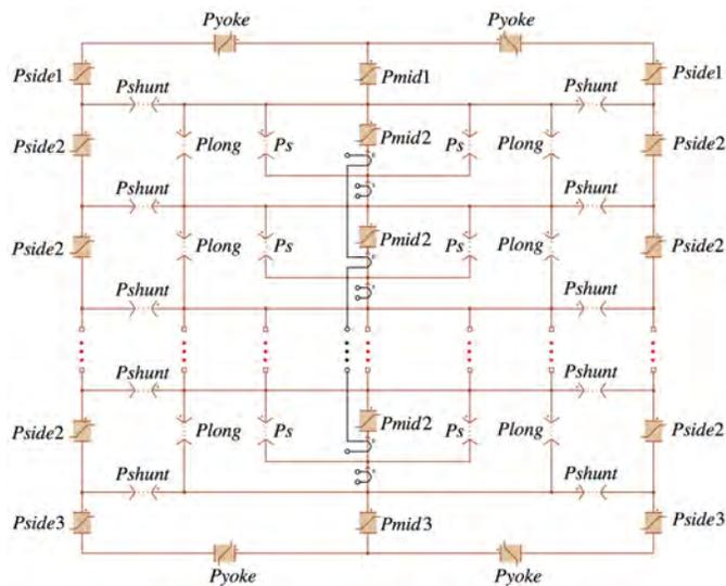
Fig. 10: Final version of the magnetic circuit model
