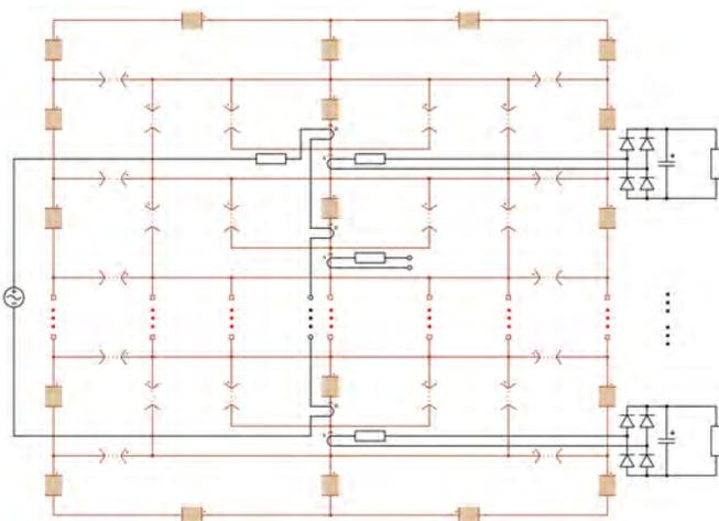
Fig. 20: System-level simulation model with diode rectifiers connected
