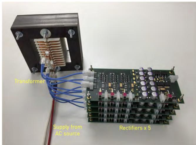
Fig. 19: Photo of the system-level verification setup
