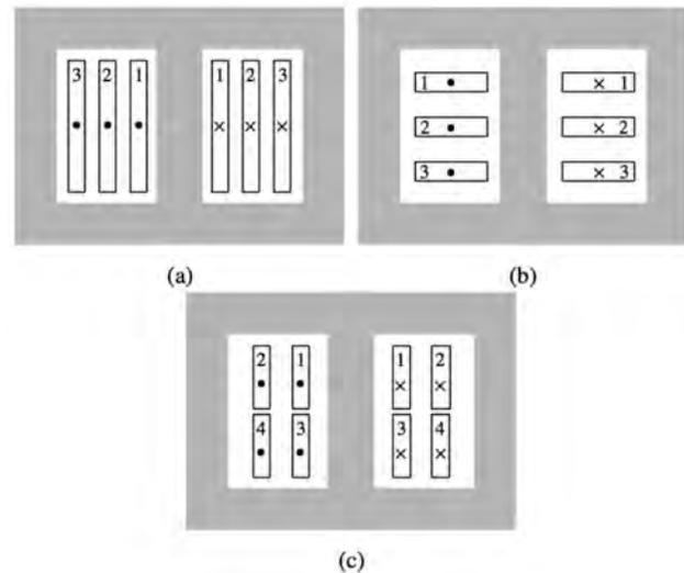
Fig. 1: Winding arrangements considered in the existing publications [9] [10] [11][13], (a) Multilayer (b) Multidisk (c) Mixed
